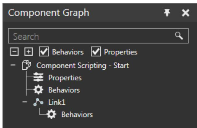
The component has one link containing the geometry of a blue platform. The platform needs to move along the X-axis of its link and be driven by a servo controller. Right now, the component does not have any behaviors and the degree of freedom (DOF) of Link1 is fixed.
