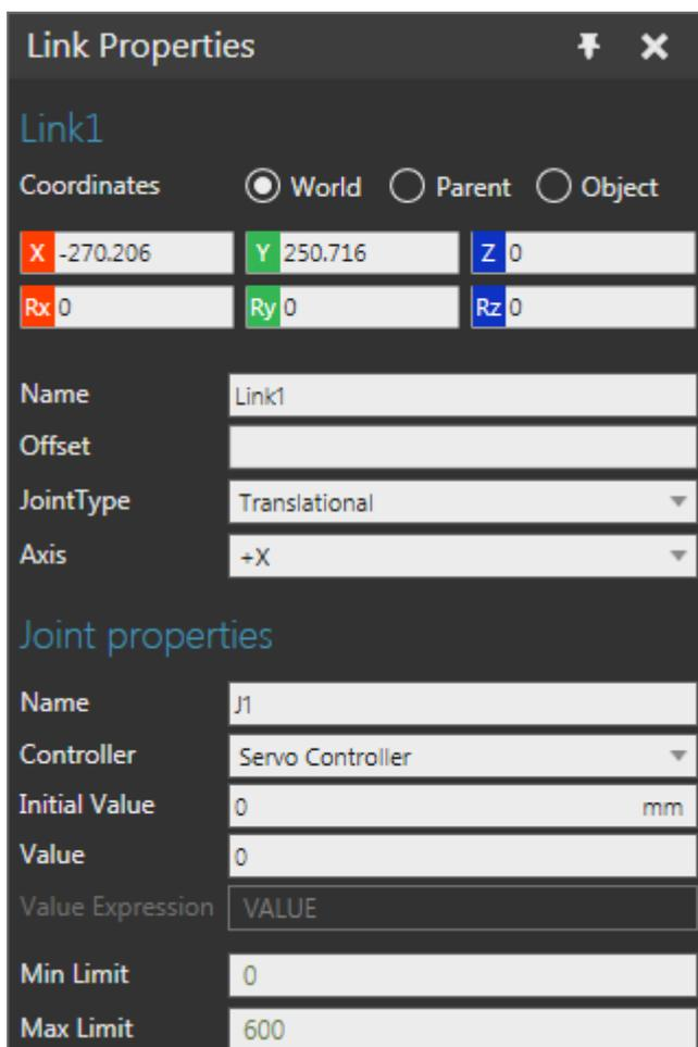
The servo controller needs additional logic to operate during a simulation. For example, the controller needs to know when to move joints, what joints to move, and how far to move them. The logic for the servo controller can be defined in a Python Script behavior.
