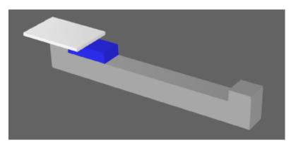
The component has a link to support the moving of parts from one end to the other via a platform. All you need to do is add the logic for moving the platform when parts reach a sensor.
