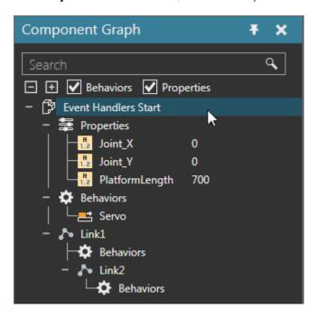
The component has two joints that can be driven by a servo controller. A component script can be used to handle events related to component properties, signals and the pulse of the servo controller.
