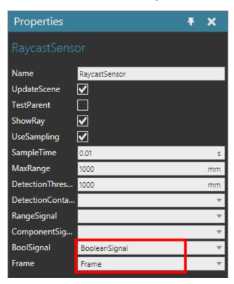
A sensor is now located at the top face center of the support base and connected to a signal. The signal value is changed every time the sensor is triggered during a simulation.
