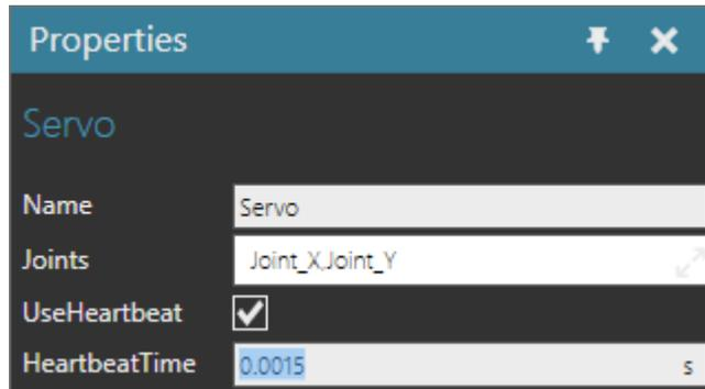
2. In the script editor, create an event handler for the OnHeartbeat event that sets the next joint targets of the servo. In this case, the event handler is used to resume the OnRun event and a global targets variable is used to store target values.
