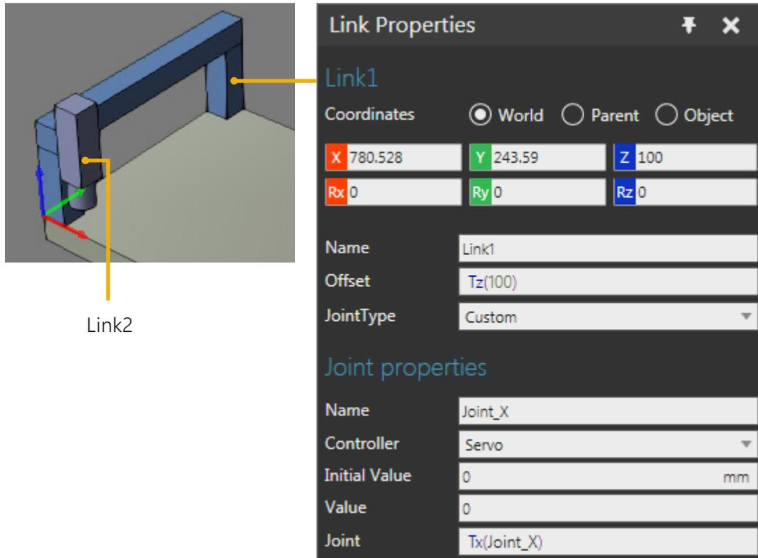
Link1 has a custom type joint named "Joint\_X" which is assigned to a Servo Controller behavior. The degree of freedom (DOF) of Joint\_X is a translational movement along its X-axis. When Joint\_X is moved it will also move the Link2 node, which is a child node attached to Link1.
