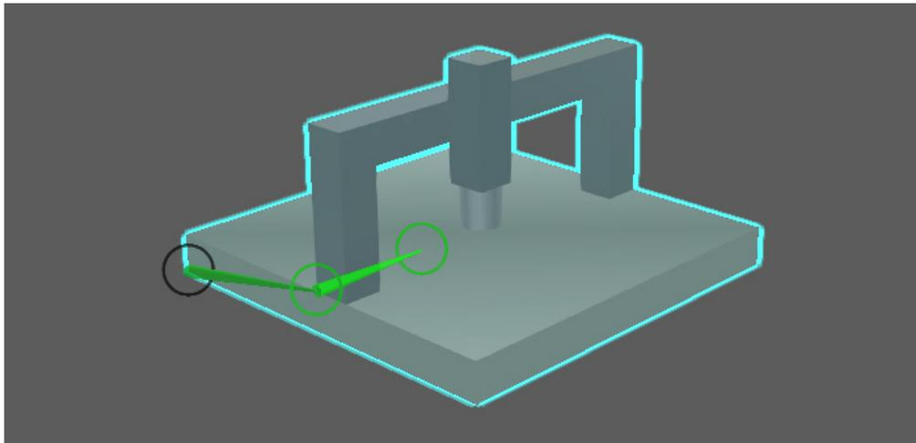
Python API can be used to control servos during a simulation. For example, you can write a component script that can manage the movements and target values of joints assigned to a servo.
