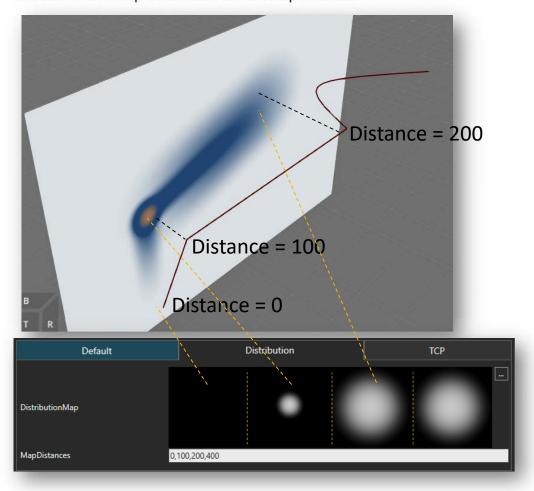
Frequency affects the paint result (how often one "layer" of paint is distributed to the surface). Faster the end effector/robot moves, more samples are needed
