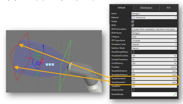
**SamplesFrequency** defines the paint distribution calculation frequency (calculation cycles per second). A higher value produces more detailed paint distribution at the cost of performance
