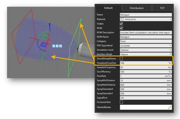
**Spray Min and Max** distance defines the minimum painting distance and the range of the paint gun
