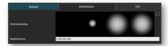
**DistributionMap** is used to define the distribution of paint in different distances from paint gun's nozzle using a bitmap. The distribution between **MapDistances** is blended.
