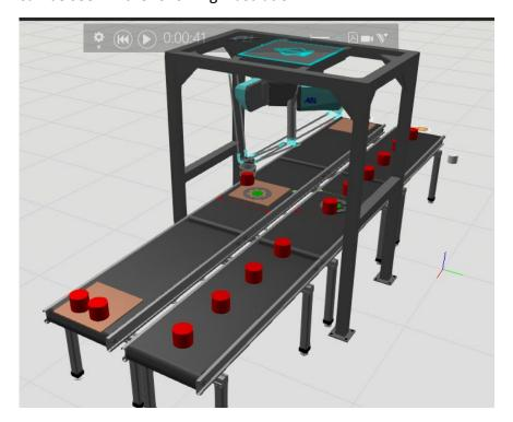
You see that conveyors move too fast for the robot and it can only pick 2 out of the 4 cylinders per tray. In this case you could either slow down the tray conveyor or make it stop. Or if you need high capacity then you can leave the conveyors as is and add a second pick area and robot.
