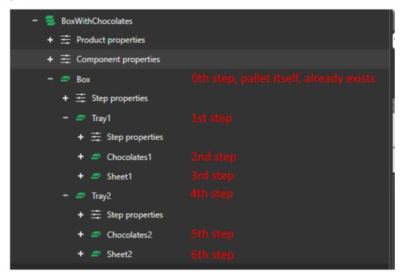
When using assembly for placing, you need to make sure that the incoming tray is already an assembly. So tray as plain product doesn't trigger transport tasks for place process. The following image illustrates an easy way to create an assembly on feeder process with the first step already included.
