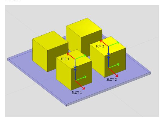
Note that in delta robots, tool frames usually have their Z-axis pointing downwards. So the default pick matrix for a product is at the center of the top surface on the product and the orientation is the product's orientation but rotated 180 degrees around Y-axis.
