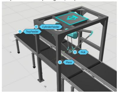
Pick process is configured to have products on conveyor and place process has products on assembly. Process filters accept any product types and processes don't stop the products. Following illustrations show the exact process properties.
