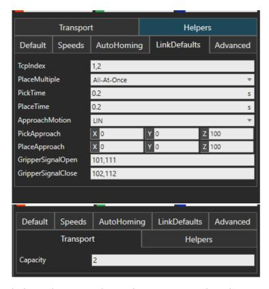
With these changes to the single gripper case, the robot now picks two products and then places them at once on the next two free slots in the assembly.
