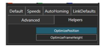
**OptimizePosition** button automatically manipulates the component's X and Y position and rotation around Z axis based on the processes that are associated with this transport controller. Before using this helper make sure to configure your process flow and associate this controller to desired transport links.
