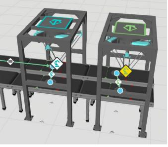
Now that we have doubled the transport capacity with the second robot, the trays get filled completely as seen in the next illustration. You could continue handling the completed assemblies and missed products downstream using standard Process Modeling features.
