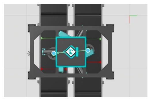
**OptimizeFrameHeight** is available when using a ceiling mount frame. Like the previous helper you need to have connected the controller to processes using transport links. When you run the helper a script will check what is the lowest reachable position with the connected robot and selected TCP (LinkDefaults::TcpIndex). Then it will check what is the lowest associated process.
