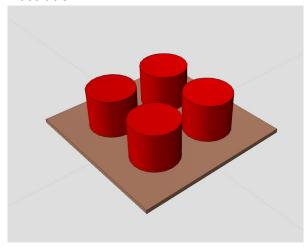
Following the common Process Modeling workflow let's define the **products** for this simulation. There's a product type for both the cylinder and the tray and these types are placed on different flow groups. In the tray flow group there's also assembly for a tray full of cylinders. In the assembly root step is the tray and its child step contains the cylinders as 4 slots.
