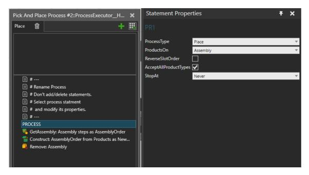
We have placed a *Pick And Place Transport Controller* over the pick and place area and it has a delta robot attached to it. **Flow** for cylinders starts from the feeder, goes to pick process and from there to place process. Pick to place transport is using the *Pick And Place Transport Controller*.
