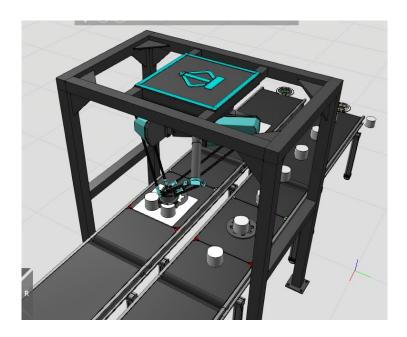
This is a manual for *Pick And Place Components* in the Visual Components eCatalog. Components are used for pick and place applications where products are moving on conveyors.
