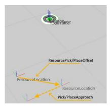
The ResourcePosition's location can be translated with the "ResourcePickOffset" and "ResourcePlaceOffset" properties in a transport link by enabling "UseCustomParameters" or by defining the default values in the Transport Controller "LinkDefaults" property tab. The defaults are applied to all links that do not use custom settings.
