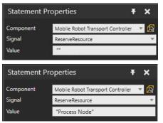
Once a Transport Controller receives the ReserveResource signal, it will reserve the next resource dispatched to transport products from/to or carry out work at the process. The value of the signal defines the process. If the value is an **empty string** (""), the caller process is used; otherwise, it must be the process **component's name** to which the reservation will be made.
