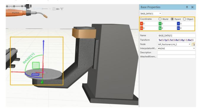
**4.** If you now return to the **Jog** panel and jog the workpiece positioner axes, the robot will move in synchronized motion along with them.
