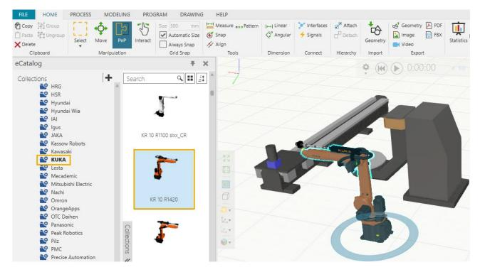
**4.** Using the **PnP** tool, bring the robot closer to the mount interface of the robot positioner. A green arrow will appear and you can then snap the robot to the positioner.
