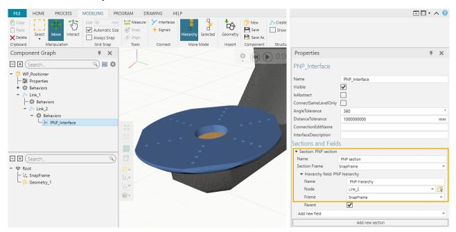
8. In the HOME tab, select the PnP manipulation tool. Then select the workpiece and hover it on top of the workpiece positioner. A green arrow will appear, and the workpiece jumps to the SnapFrame location that was created.
