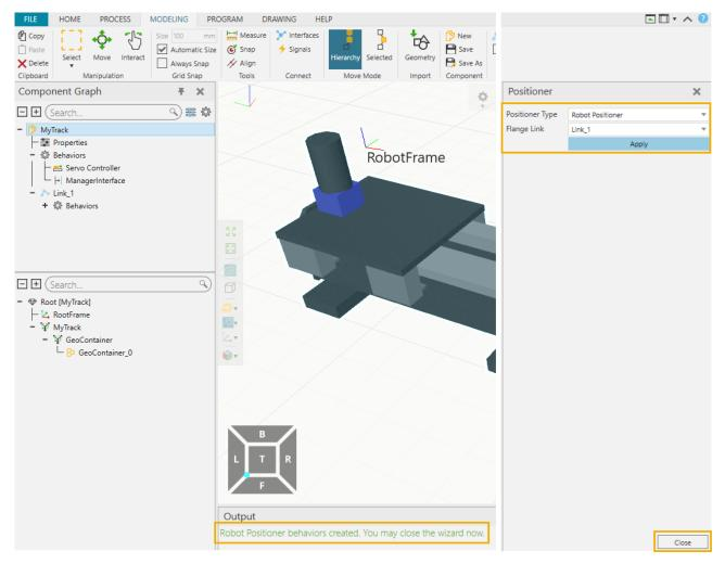
**4.** The wizard will create a **MountInterface** behavior and a **RobotFrame** property that is used to connect the track to the robot.
