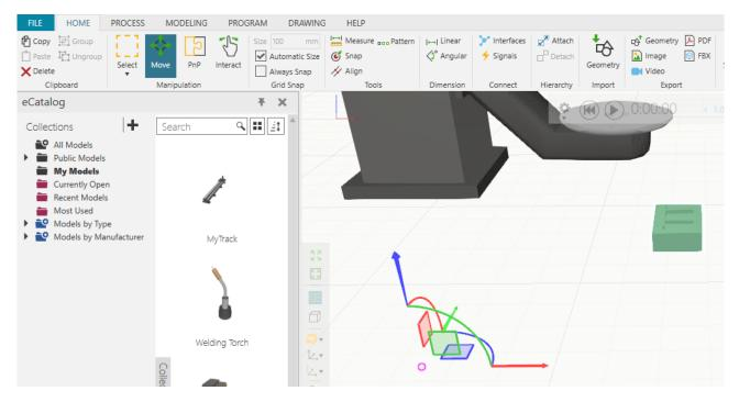
2. To move the workpiece correctly in the 3D world view, it's better to place the origin somewhere at the base of the component and in a position where it is easy to snap it to the workpiece positioner. Let's begin by rotating the component so we can see its base.
