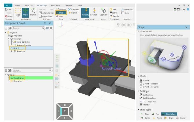
6. The position of this RobotFrame will be the position the robot component will later snap to when using the PnP mode. And to position the robot correctly, in Feature Properties on the right, with Coordinates set to Object we can rotate the Rz axis by -90 degrees.
