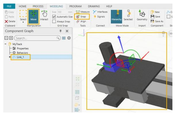
**3.** With **Coordinates** set to **Object** in the **Link Properties** on the right, we must make sure that the link is oriented so that the Z-axis is pointing upwards and the X-axis is heading along the track.
