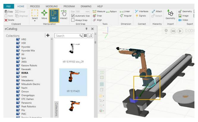
5. If we now select the **Interact** tool and jog the pedestal on the track, the robot moves along with it the track.
