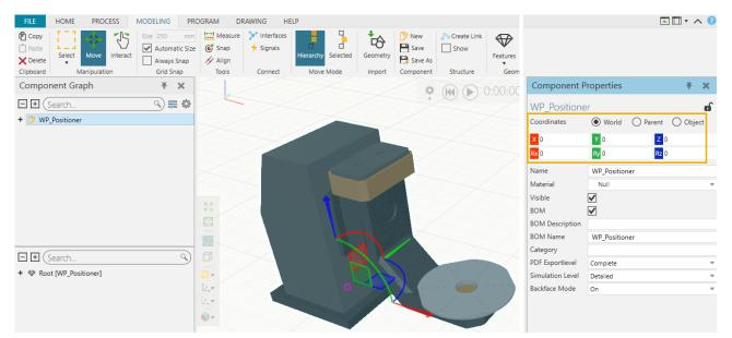
Tip! To quickly reset the **Coordinates** to **0**, you can click on the red X, green Y or blue Z axis controls.
