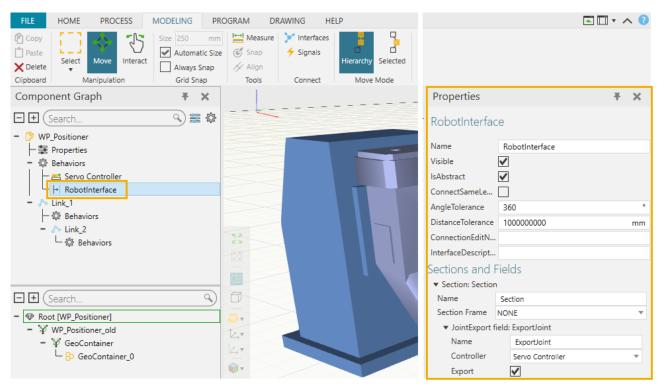
**4.** In this example the imported workpiece positioner component already has materials assigned to it. If materials are not present, then you may assign materials to the component.
