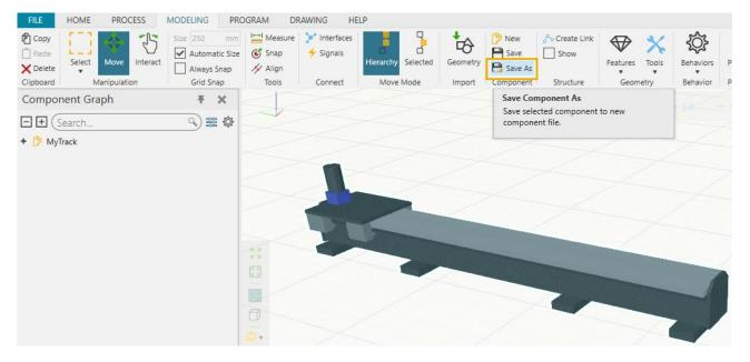
2. In the Save Component As panel, set the Type to Robot Positioners and then click Save As to save the file to your computer. For example, you could save it to your My Models folder so you can access it easily from the eCatalog.
