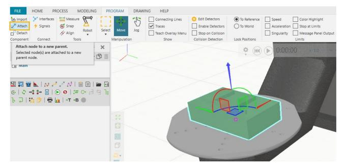
2. Hovering the mouse over the workpiece positioner, a red bounding box appears which you can use to select the last link of the workpiece positioner. Note the messages that appear in the **Output** panel below.
