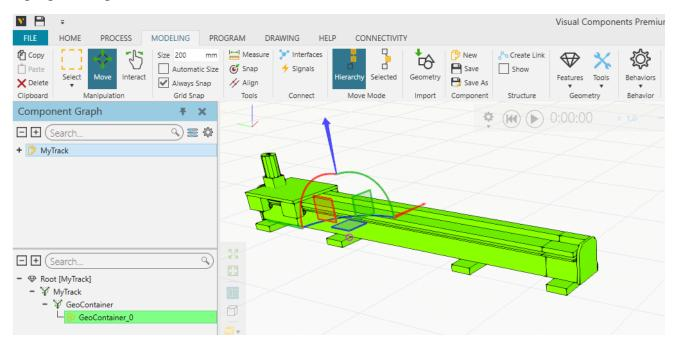
Select the Link\_1 we created on the left, then select the Move tool from the Manipulation group, and use the Snap tool to snap the position of the link to the center of the track mount plate.
