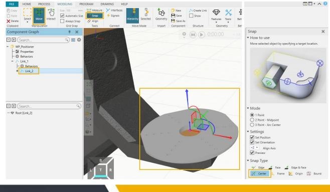
6. With Coordinates set to Object in the Link Properties on the right. We must make sure that Link\_1 and Link\_2 are oriented so that both axes rotate around their Z-axis.
