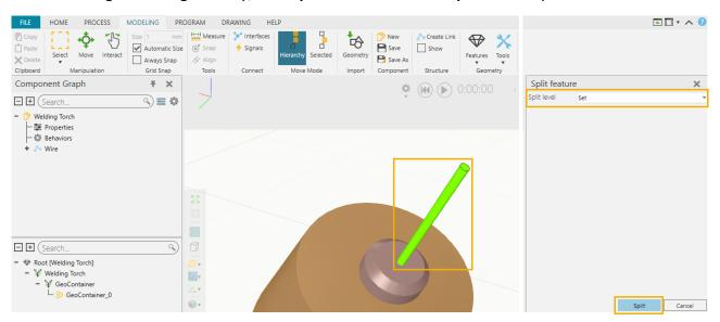
**3.** Then from the **Tools** group in the ribbon, select the **Measure** tool and measure the radius of the wire, noting the results that appear as *Measurement Length* in the **Output** panel below.
