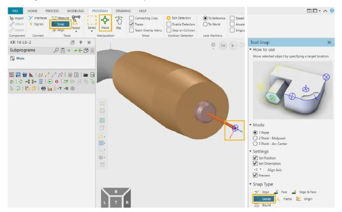
**4.** In the **Tool Properties**, with **Coordinates** set to **Object** check that the Z-axis is pointing outwards, and the X-axis is pointing towards the robot.
