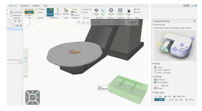
2. Now hover your mouse over the workpiece positioner. You can see a preview of where the workpiece will be snapped on the workpiece positioner. Then left mouse click after choosing the correct target location.
