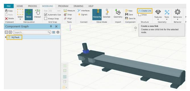
**Note:** When the **MyTrack** component is selected, in the **Component Graph** the whole component is selected and it will then appear highlighted in blue. If you select only the geometries from the Node Feature Tree below, the selected geometries will appear highlighted in green.
