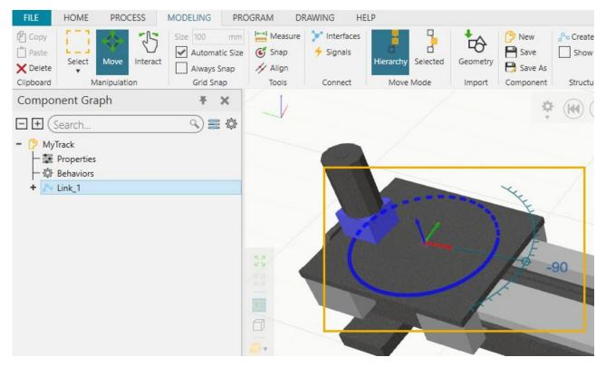
**Note:** For links and components, always check their orientation with **Coordinates** set to **Object**.
