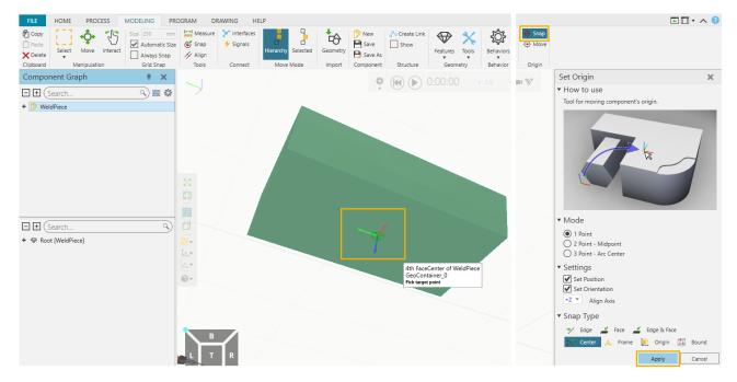
4. If we now check the component using the **Move** tool, in its **Component Properties** with **Coordinates** set to **Object**, we can see that the origin should be adjusted to match the workpiece positioner we will attach it to.
