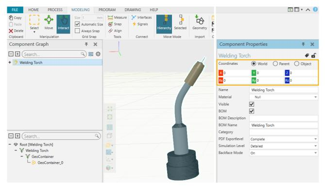
Tip! To quickly reset the **Coordinates** to **0**, you can click on the red X, green Y or blue Z axis controls.
