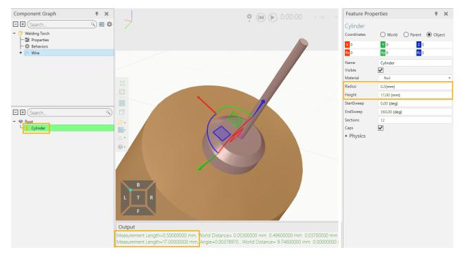
7. Then from the **Component Graph** on the left, select the **Welding Torch** component and from the Node Feature Tree below, under the **Root** select the **Geometry** of the original wire, right-click on it and click **Delete** to remove it.
