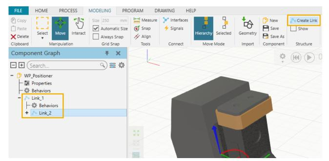
4. Select the Link\_1 we created in the Component Node Tree on the left and then select the Move tool from the Manipulation group in the ribbon and use the Snap tool to snap the position of the link to the first joint of positioner.
