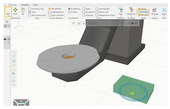
2. Then in the **MODELING** tab, select the workpiece positioner link where you wish to create the interface the workpiece will snap to using PnP.
