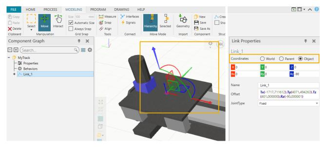
Tip! If you place your mouse cursor close to the degree indicators that appear, you can rotate the axis in increments of five degrees to set an exact value of e.g. 90°.
