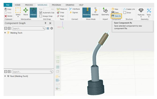
2. In the **Save Component As** panel, save the welding torch component in the same manner as the previous components, except here the **Type** would be **Tools** or **Robot Tools**.
