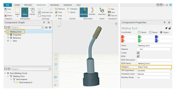
2. In this example the imported torch component already has materials assigned to it. If materials are not present, then you may assign materials to the component.
