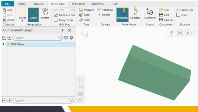
**3.** Then in the **MODELING** tab, from the **Origin** group select **Snap**. Then snap the origin, for example at the center of the base of the component and click **Apply**.
