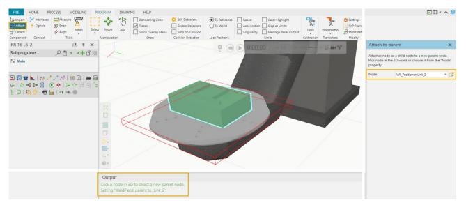
**3.** So now if we **Jog** the robot, when the workpiece positioner moves the attached workpiece will move with it.
