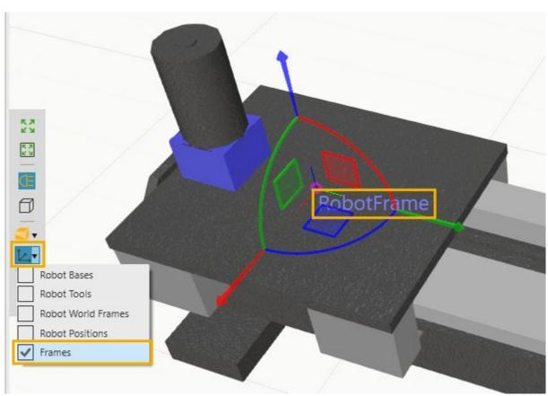
**Tip!** Enabling **Frame Types** and then **Frames** from the 3D World Toolbar allows you to visualize the Frame names in the 3D world view.
