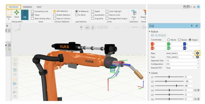
2. A Base Properties panel will appear. By default, the node would be **\*WORLD\***. Click on the yellow pick property control and choose Link\_2 from the workpiece positioner
