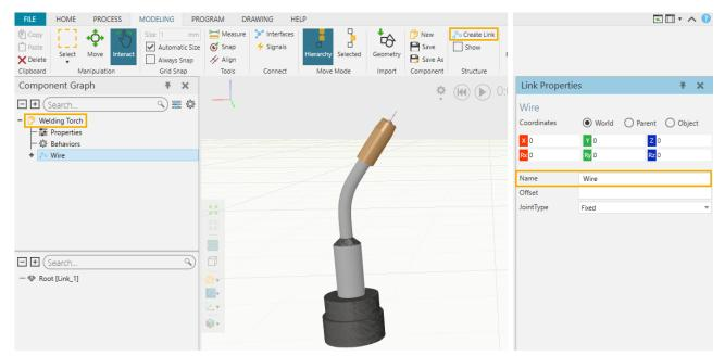
**3.** Select the **Wire** link on the left, then select the **Move** tool from the **Manipulation** group and use the **Snap** tool to snap the position of the center point of the base of the wire.
