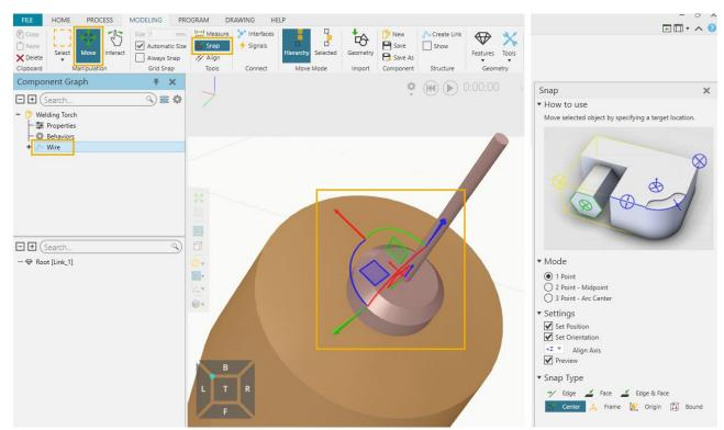
**4.** With **Coordinates** set to **Object** in the **Link Properties** on the right, we must make sure that the link is oriented so that the Z-axis is pointing upwards.
