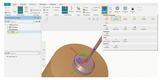
If we have placed the wire link correctly, the wire should appear in the correct location. Then in the Feature Properties of the new Cylinder component, set the Radius and Height to the *Measurement Length* values that appear in the Output panel e.g. 0.5 (mm) and 17.00 (mm).
