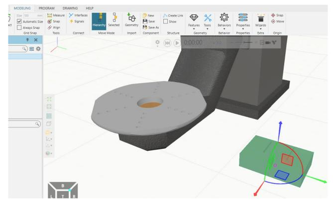
2. Then rotate the camera view so we can see the base of the workpiece. Then from **Tools** click on **Align**. We will select **Snap Type** as **Center** and select the center of the base of the workpiece as the first alignment point.
