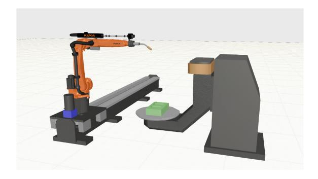
Learn to model robot positioners, workpiece positioners and welding torches for OLP use and then use these options to setup a functioning layout.
