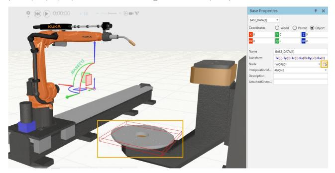
**3.** Now set the **Coordinates** to **Parent** and reset all the X, Y and Z values to zero so that the frame is in zero location with respect to the parent frame (which in this case is the workpiece positioner plate).
