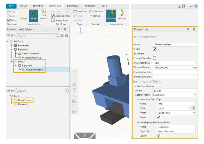
Select the Link\_1 in the Component Node Tree on the left. And then from the Node Feature Tree below select RobotFrame under the Root, and using the Snap tool, snap it to the center of the track mount plate.
