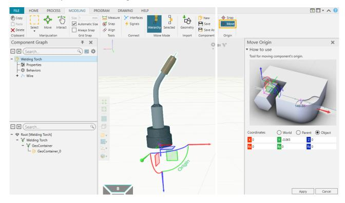
7. In this example in Move Origin with the Coordinates set to Object, we will rotate the Rx axis by -180 degrees and then click Apply.
