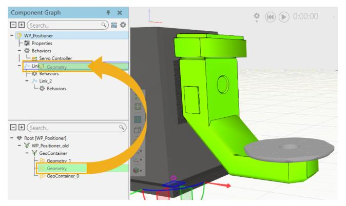
And holding the Shift key, left mouse click on **Geometry\_1** and drag it up placing it under **Link\_2**.
