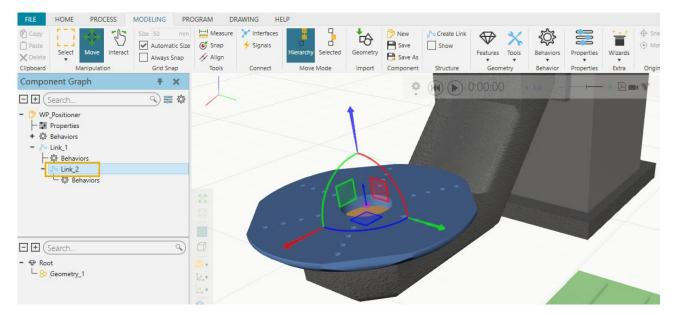
3. From the Features menu in the ribbon select Frame which will create a Frame under the Root in the Node Feature Tree for Link\_2.
