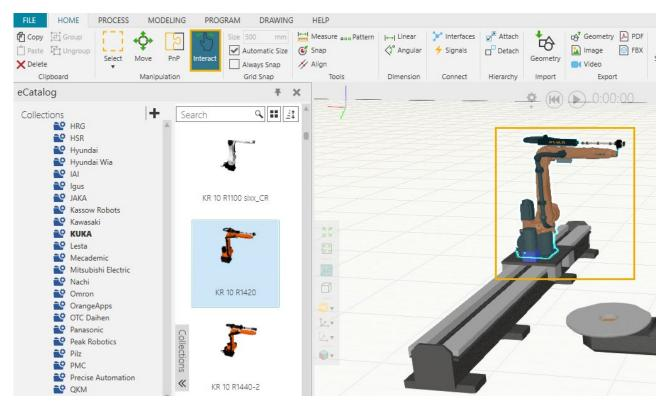
**6.** We should now connect the interfaces between the robot and the workpiece positioner. Click on **Interfaces** and select the robot to see its interfaces.
