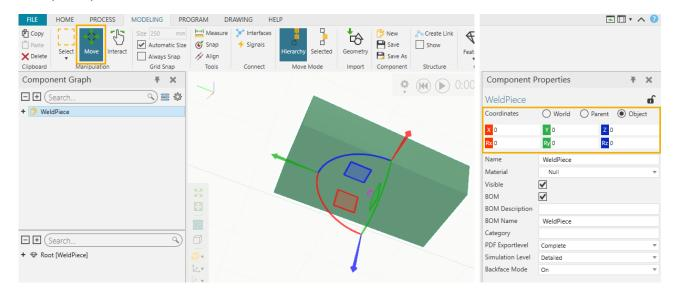
5. So then using the Move Origin tool, in Move Origin with Coordinates set to Object, we will rotate the **Rx** axis by -180 degrees and then click **Apply**.
