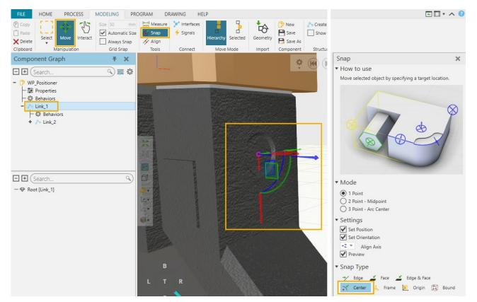
5. Then select Link\_2 and using the Snap tool again, snap the position of the link to the center of the workpiece positioner plate.
