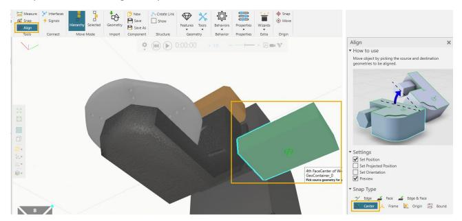
**3.** Then with **Set Position** enabled in the **Align Settings**, pick the second point for alignment on the surface of the workpiece positioner. And then click to **Close** the **Align** panel.
