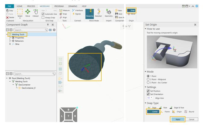
6. And if necessary, use the Move Origin tool to rotate the frame.
